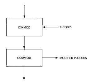
Fig. 2. Flowchart showing the general flow of data and programs necessary to change the byte-sex of a Pascal disk unit containing p-code files
